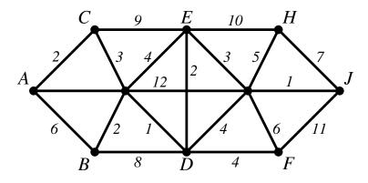
(a) Apply Dijkstra's Algorithm to this graph, where the starting vertex is *A*.
