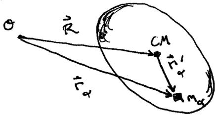
a rigid body and define  $\vec{r}'_\alpha$  as the position of  $m_\alpha$  w.r.t. the C.M.
