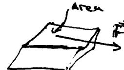
Strain is the <sup>fractional</sup> change in shape P3/3 or deformation due to a stress
