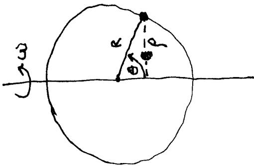
The bead is constrained to move along the wire. In particular if you know  $\theta(t)$  then you can find  $x(t)$ ,  $y(t)$  and  $z(t)$
