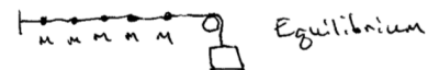
Figure 1: A collection of N masses, each of mass m , at equilibrium under a tension T .
