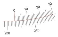
Vernier scale reading an angle of 232° 46 ' (232 degrees, 46 minutes), or 232 + 46/60 = 232.766667°.
