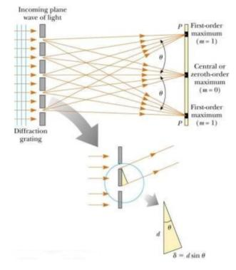
2. Use the result for d from 1. to calculate the wavelength of at least 5 different color spectral lines from a mercury lamp. Again average the angles for corresponding orders. For each color you should find the wavelength from at least 3 different orders if possible. Use these measurements to find the average wavelength and standard error of each color. Compare your results with values for spectral lines in mercury found at
