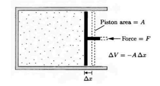
Let's consider the compression of a gas at fixed pressure, with that process and constraint we have the total work is
