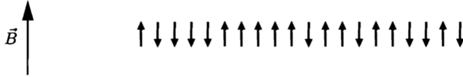
Figure 2.1. A symbolic representation of a two-state paramagnet, in which each elementary dipole can point either parallel or antiparallel to the externally applied magnetic field.
