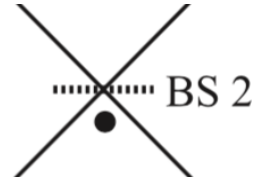
Figure 3: A beam splitter with the silvering indicated explicitly by the \bullet .
