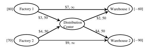
On each edge, the first number is the cost and the second number is the capacity.
