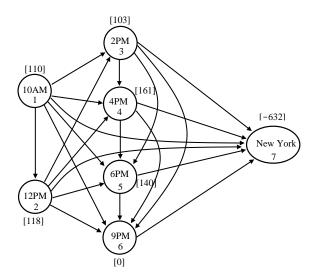
The net flow through each vertex is labeled in the graph. A Minimum Cost Flow problem needs to also have two labels on each edge: the cost and the capacity. As it would be hard to put these labels on the above graph (since it is already so complicated), the costs and capacities are shown in the following tables:
